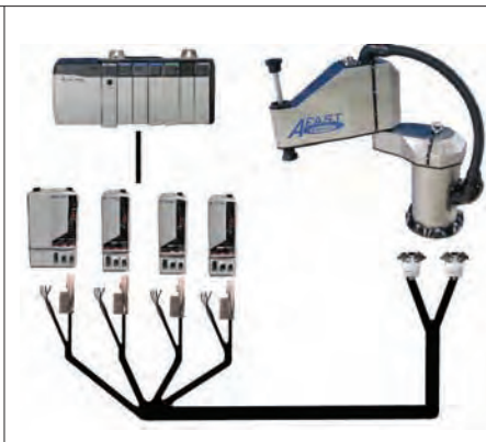
Rockwell Automation Encompass Partner AFAST Robotics' SCARA robots include one cable that contains four encoder cables and four power cables at optional lengths.
