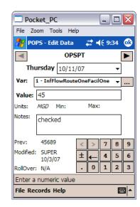
Pocket OPS allows you to use your Windows Mobile PDA to collect data in the field. Plan a route...walk the route... download the data. The screen will alert if limits are exceeded, show yesterday's value and do calculations.
